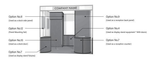
System panels are basically plywood panels with PVC vinyl color sheet finish.
